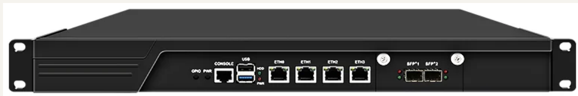
FC-X2-SRV-1U front panel — console · USB 3.0 · ETH0-ETH3 Gigabit · SFP1-SFP2 fibre · power and HDD indicators
